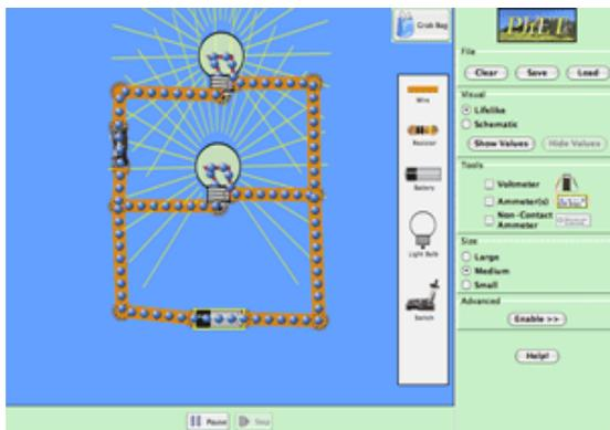
*Circuit Construction Kit*: An electronics kit in your computer! Build circuits with resistors, light bulbs, batteries, and switches. Take measurements with the realistic ammeter and voltmeter. View the circuit as a schematic diagram, or switch to a life-like view
