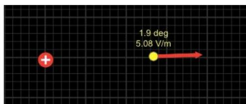
6. Move the sensor away from the point charge along a major grid line and use the **tape measure** tool to make five distance field strength measurements
