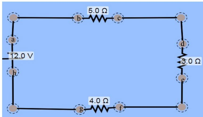
2. Connect the positive terminal of the of the voltmeter to point **h**, and then touch the labelled points in turn, noting and recording the reading on the voltmeter in each case. Calculate, by subtraction ( $V_b - V_a = V_{ab}$ ), the potential difference across the power source and across each load and conductor. Remove the voltmeter from the circuit.
