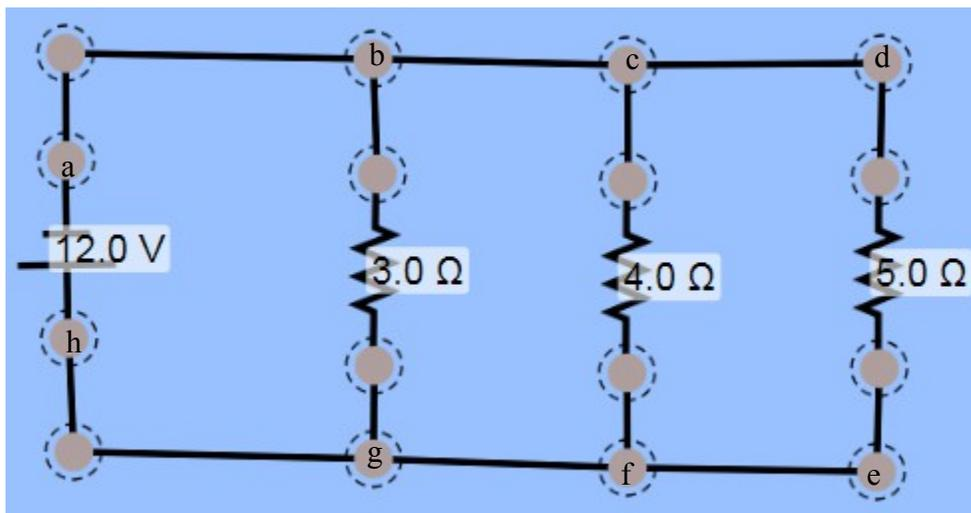
2. In the same way as before, by connecting the positive terminal of a voltmeter to point **h** and then take readings of electric potential at each point, and then calculate by subtraction ( $V_b - V_a = V_{ab}$ ) the potential difference across the source and across each load and conductor.
