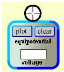
It is used to find the value of the potential at any point in space and plot the lines of equipotential in the area. The circle at the top changes color to reflect the relative magnitude and polarity of the potential at the point in the cross hairs. You will be using this tool to plot the potential lines.
